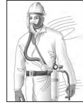
Supplied Air respirator (SAR) with an auxiliary escape bottle (FF-PD) (1,000 APF)
