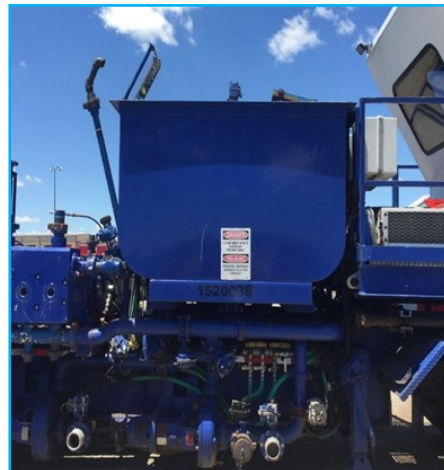
Coil Mixing Tub
