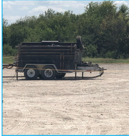
Mobile Blowdown Tank
